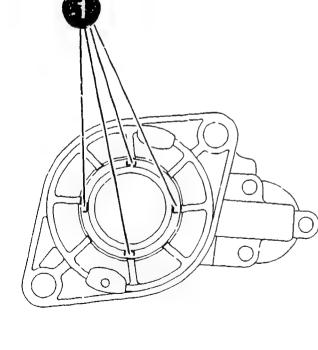
COMPONENT CHECKING AND REPAIR Checking drive-end shield (version with bushing) Installing bushing: Use mandrel of mandrel press to carefully flush-fit bushing in drive-end shield from inside. ATTENTION: Pockets of new bushing must be completely filled with grease.
